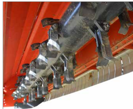
Special hammer design or fan or universal blades creates a suction effect lifting material and improving cutting.
