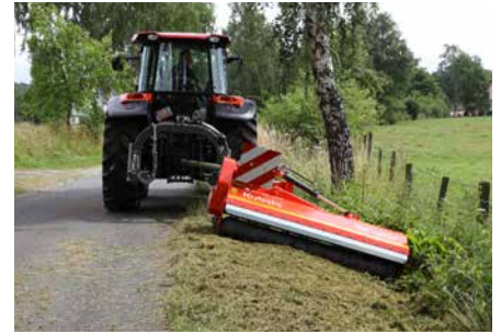
It banks down to an angle of -65 degrees.
