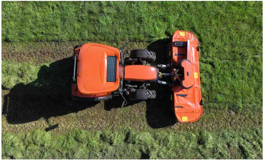
DM4032S Compact with gravity point close to the tractor is an important feature when operating in hilly conditions with smaller tractors.
