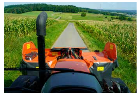
Narrow transport position with good visibility. Hydraulic foldable guards are available as option.
