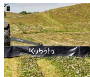
To avoid driving on mown grass, a swath forming kit is optionally available for 3036 and 3040.
