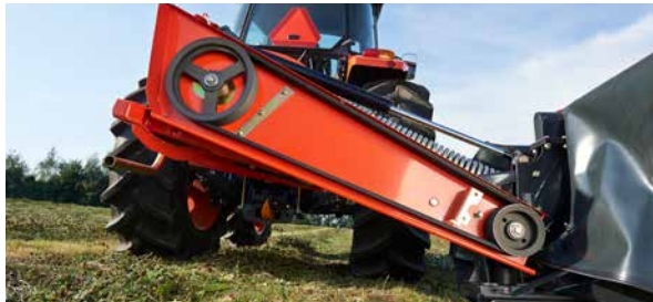
Four v-belts ensure excellent transfer of power.
