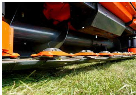
Crop is guided towards the centre by auger and closed guide plates.
